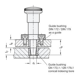
The length I<sub>7</sub> is determined by the penetration depth of the indexing pin into the cone of the bush.
